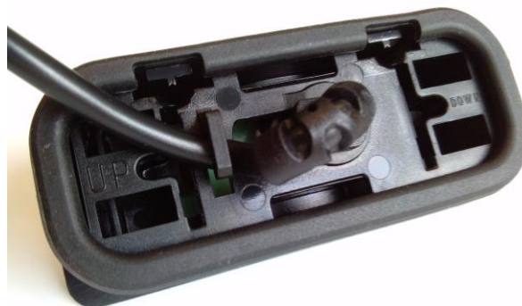
Figure 4: The text "UP" and "DOWN" indicate the movement direction of each button to prevent wrong mounting
