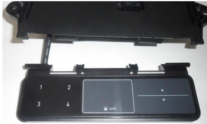
Figure 8: the user interface panel released from the fixed part in case of too high forces applied to it
