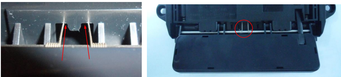
Figure 9: left: springs inside the sliding mechanism: right: springs are in place
