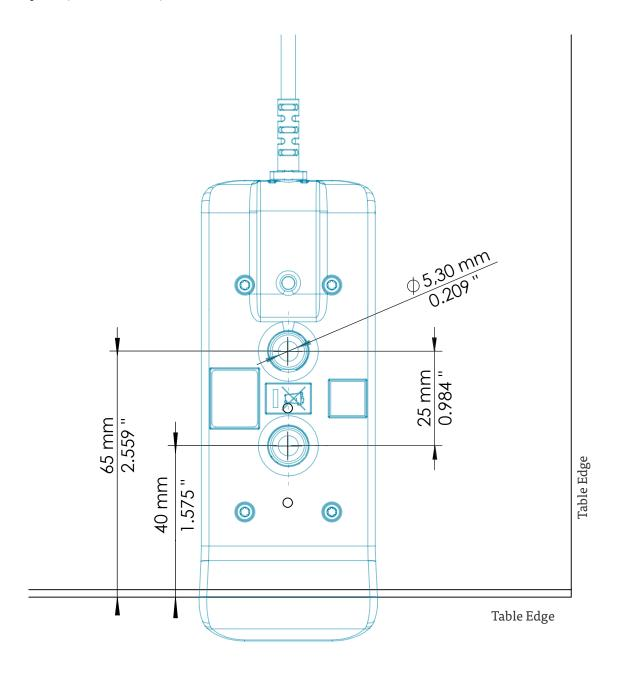
Fig. 3: Drilling Template, EASY2move
