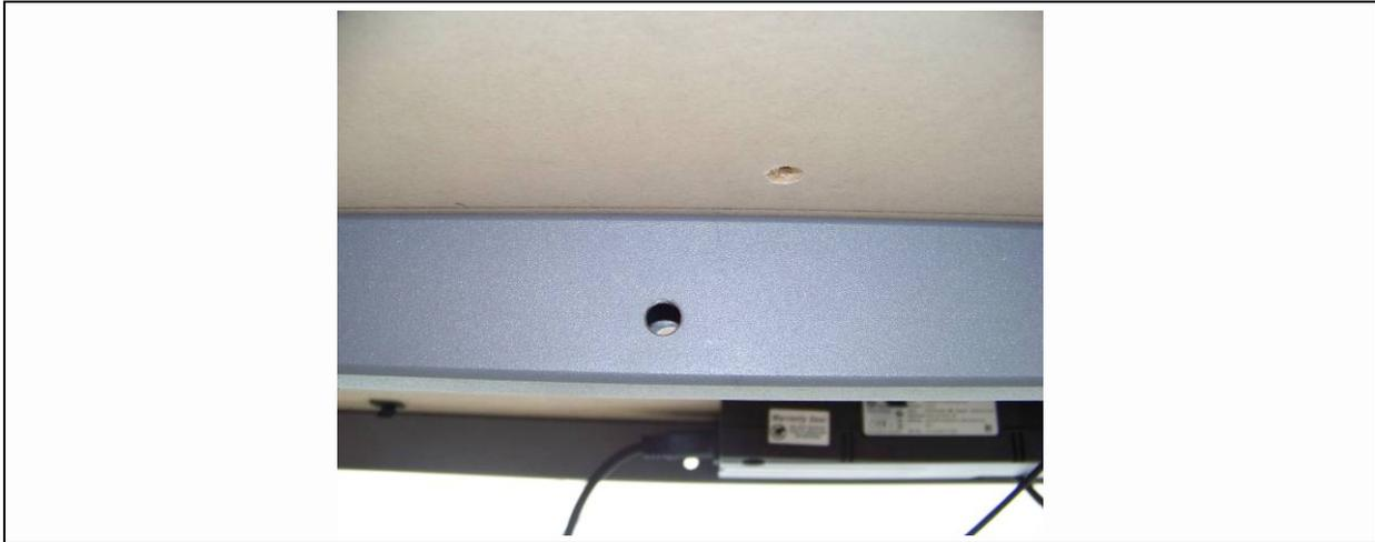
Figure 3: Mounting holes for the sensor unit
