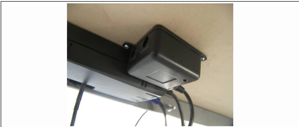
Figure 5: ACS-CB-SENS mounted near the motor control unit
