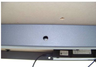
Fig. 4: Drill holes for the assembly of the sensor unit
