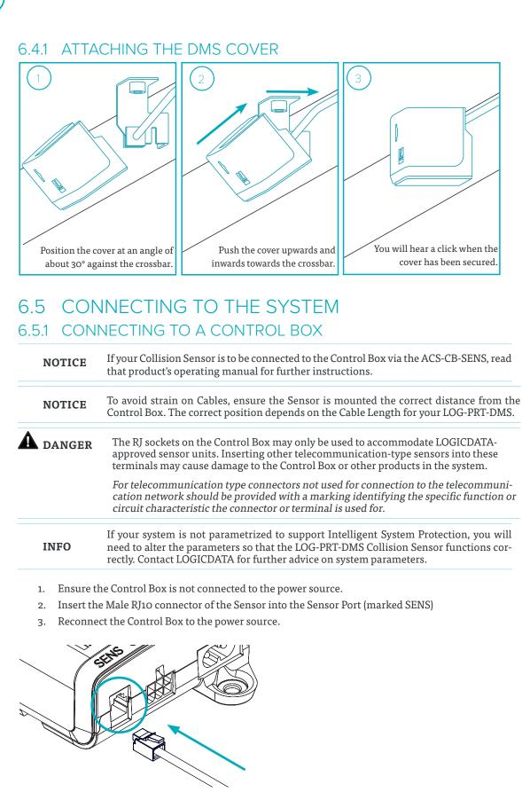
Fig. 5: Attaching the Sensor Adapter Cable to an Example Control Box
