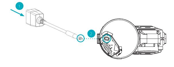
Fig. 6: Attaching the Sensor Adapter Cable to the DMG90
