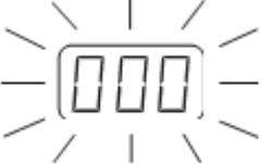
If **000** flashes on the display, a reset is necessary. This procedure is explained in section 4.2.4.
